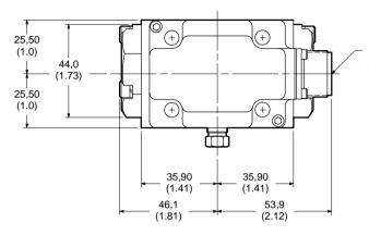
Electrical connector mates with MS-3106-14S-2S (4 pin). Plus signal to A or C causes flow out of port B.
